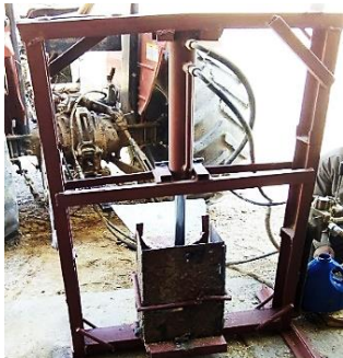
Figure 1 feed block production machine, designed and built by the researcher
